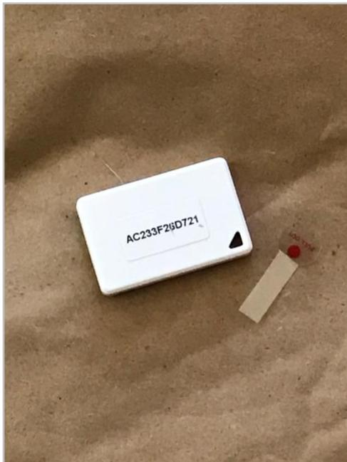
Remove the plastic strip attached to the beacon, which enables the battery.
