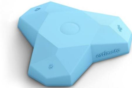
This product is meant for developers and works with the Estimote's Events API. The unit runs javascript microapps on the device itself, and can call code for those apps from the cloud via the cellular network. In addition to the button functionality that is described earlier in this video, you can program this device to act as a GPS tracker or a BLE gateway.
